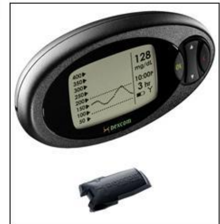
Dexcom STS 7 Continuous Glucose Monitor Sensor and Receiver. Courtesy of Dexcom.
